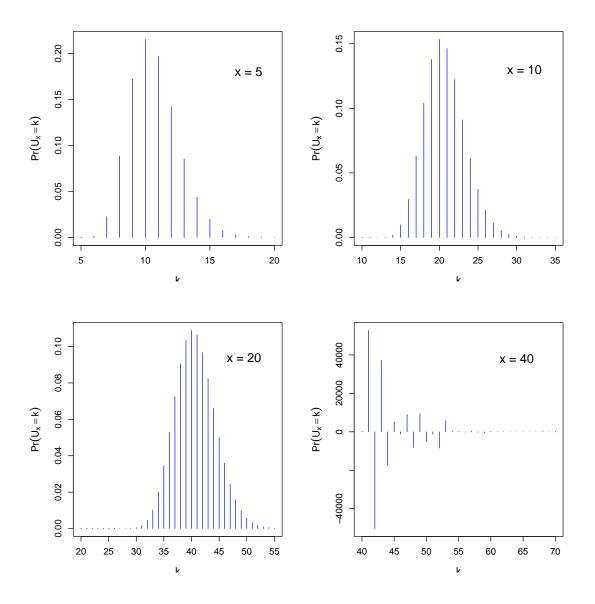
The problem is the well-known instability that often arises when calculating alternating sums with standard double precision arithmetic. Although the problem is clear at x = 40, it first arises for much smaller x and can be identified by the occurrence of negative 'probabilities'. For example, with x = 14, the smallest value obtained is  $-1.2159 \times 10^{-10}$ .
